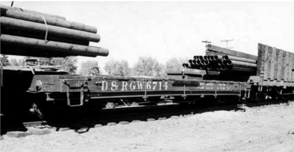
Two modified gondola cars carrying fifty-foot lengths of drill pipe are coupled astride D&RGW Idler Flat 6714 in Alamosa, July, 1956.
