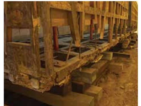
The two end platforms were far beyond saving and were scrapped to prepare for leveling the car.
