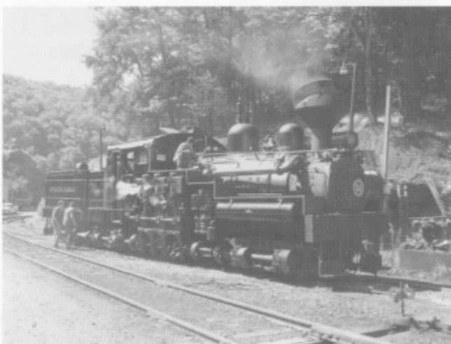
Shay No. 11 is prepared for its morning trip. This large, 103 ton, Shay is the only Pacific Coast type Shay in the eastern U.S. It was moved to Cass from California in 1997. (David Lee)
