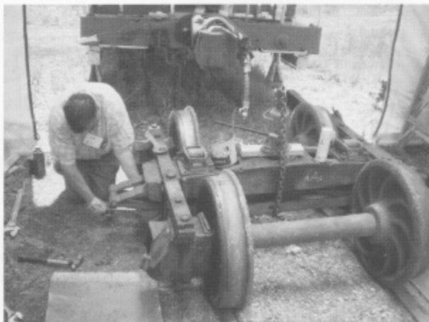
Chuck Everitt in the process of completely tearing down a truck for 0503.
