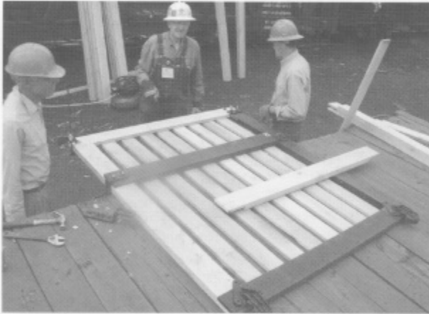
George Detwiler, Mike McGinley, and Scott Hardy rebuild one of the doors for Stock Car 5549.
