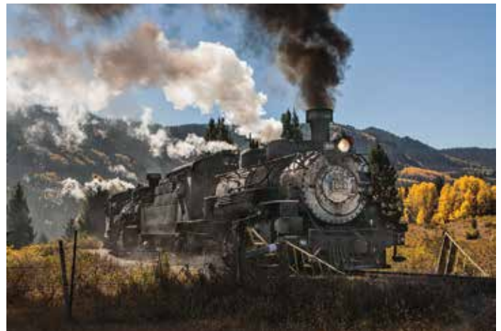
A doubleheader climbs the pass in the Fall of 2017. Because of the assistance from 489, Lead Locomotive 484 doesn’t need to work as hard and thus puts out fewer cinders. There is a “bonnet” on the stacks on both locomotives. Photo: Chris James
