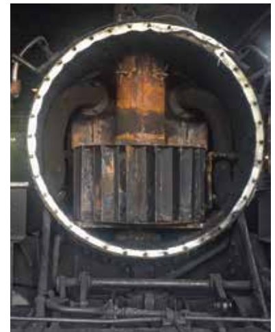
A “cyclone” cinder catcher in each smoke box breaks up large cinders before they can escape. “Bonnets” on the stack capture smaller cinders. Photo: John Bush
