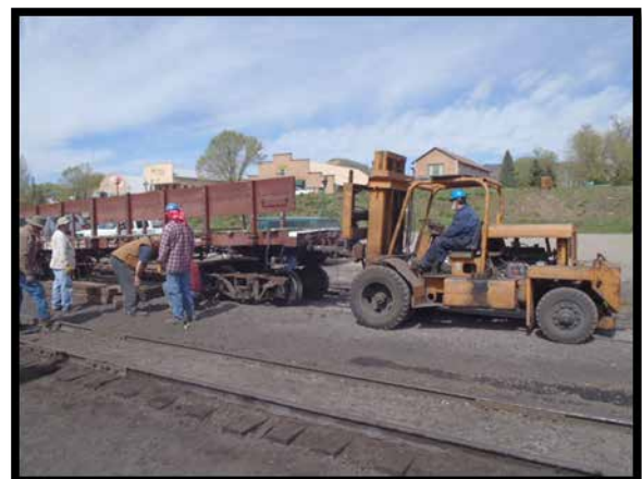
Wheel sets being changed out on the Cinder Bear Gondola
