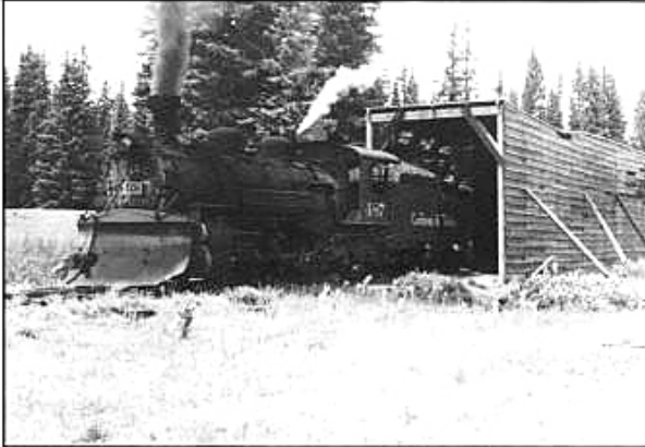
Engine no. 487 pulls a flatcar with tools and unused construction materials from under the Cumbres snowshed at the end of the work sessions. Note completed siding on the east side of the snowshed. August 1993. Photograph by Terri Shaw.
