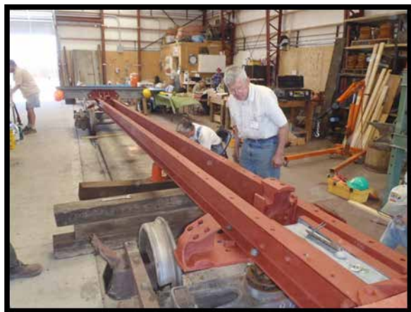
TL Bill Pratt examines frame newly coated with red oxide primer
