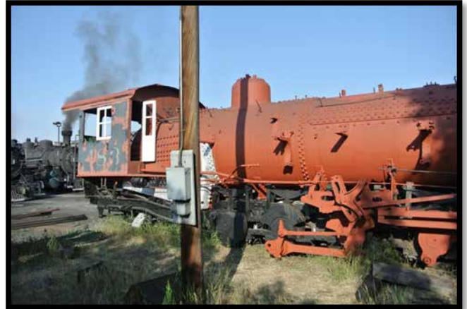
Engine 483 at the end of Session D shows a door and window installed
