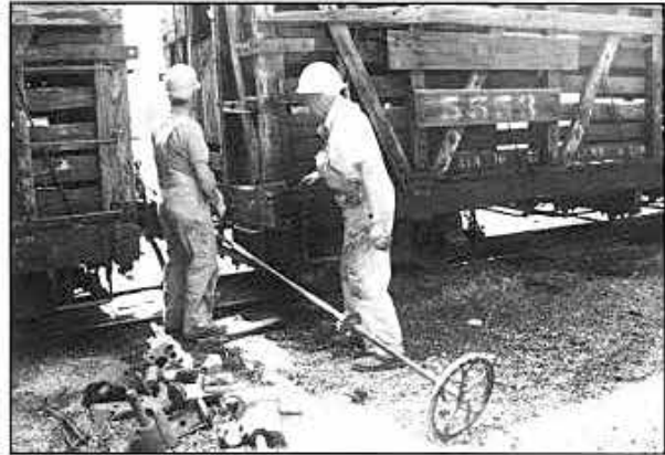
At Chama the brake rigging was reattached to one of the double-deck sheep stock cars donated to the railroad by the Friends. The brake linkage was disconnected years ago when the car bodies were separated from their trucks. July 1993. Photograph by Jessica Ratliff.
