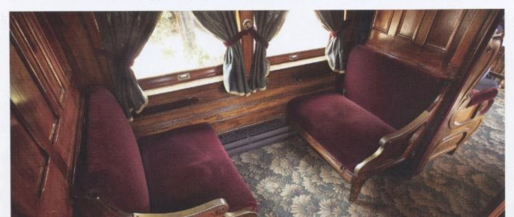
The pullout berth in the observation room gets made up when the seat cushion is pulled forward far enough to allow for the lowered seat back to become the rest of the berth. Having the heating pipes under the berth must have been a plus when the snow flew up in the Rockies. COURTESY OF STEVE GILLARD & RICHARD HARRIS
