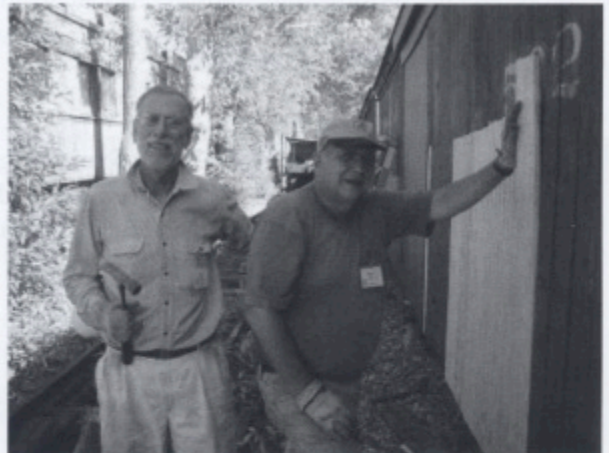
Ronald Schaefer and TL Roger Breeding finished splicing in new wood siding on the F&CC box cars.
