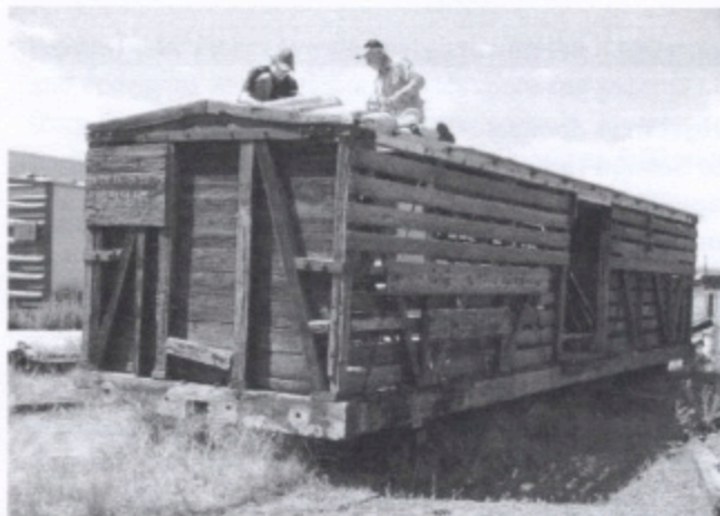
Matthew Myers and Kevin Corwin installing roof decking.
