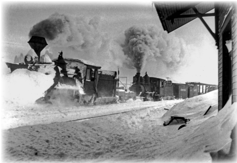
Westbound snowplow and flanger helping freight at the depot. From the Richard L. Dorman collection. File no. RD013-022
