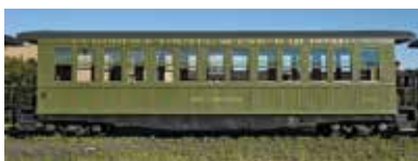
C&TS Coach 503 Rebuilt on 6500 series flat car, 1982
