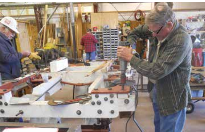
Additional bracing was placed on the corners of the 053 truck.
