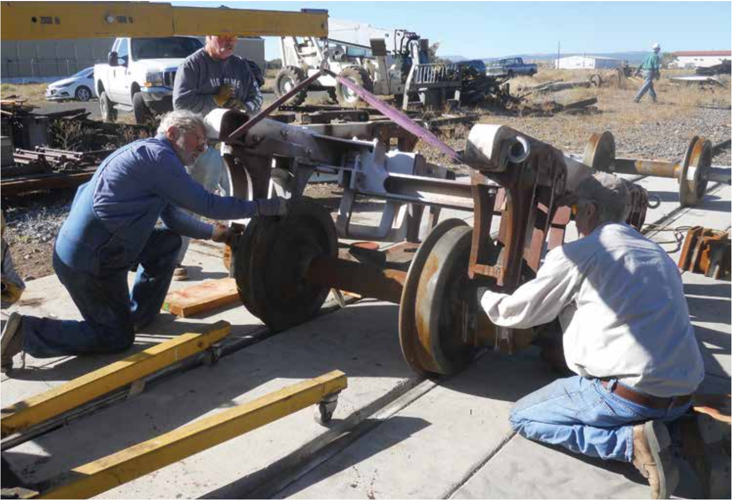
Above: The completed frame and pedestals are lowered onto wheel sets. Below, left: Journal boxes are fitted into the pedestals.
