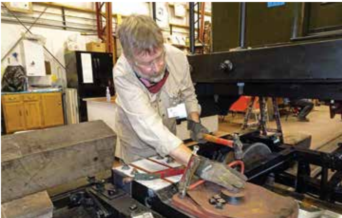
Painted, the final height of 470's bolster still needed adjustment.
