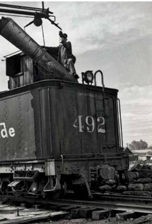
1958 Top: K-37 2-8-2 492 rides the turntable in Alamosa. Bottom: In the Alamosa engine terminal, a hostler fills 492's tender from a standpipe, then the locomotive heads for the coaling station.
