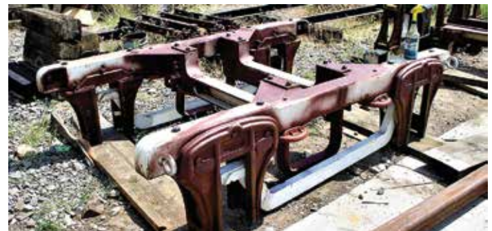
Top: Truck assembly has moved outside the CRF. Bottom: Assembly complete, the frame awaits wheel sets.
