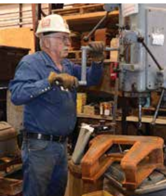
Chuck Dueker prepares to drill mounting holes in a pedestal.
