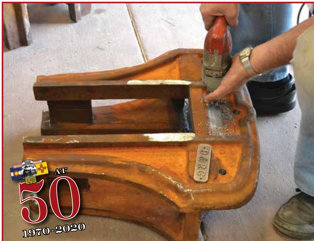
Finishing touches, with attention to detail. The late John Weiss drills holes to install a D&RG nameplate on a pedestal destined for RPO 65. D&RG and Pullman plates were created and cast by Weiss for the restorations. For a close-up of the nameplate, see page 9. Photo by Don Atkinson
