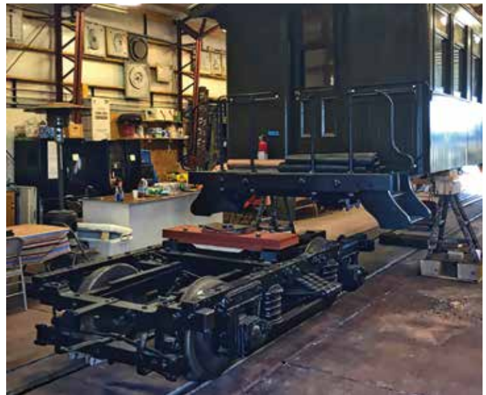
Completed, 470's trucks are ready to roll! Some of John Weiss' casting patterns adorn the far wall of the CRF.
