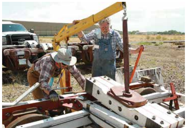
A bolster is lowered into place on a truck for Pullman 470.
