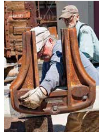
Pedestals attach to the frame.
