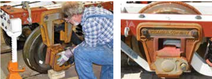
Above: The completed frame and pedestals are lowered onto wheel sets. Below, left: Journal boxes are fitted into the pedestals.
