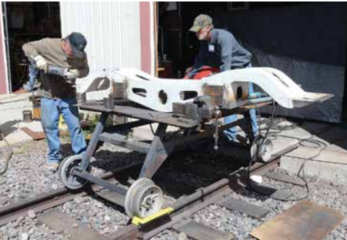
With the welding done, welds are ground to perfection.
