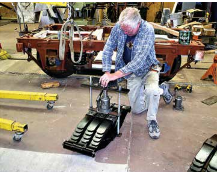
Russ Hanscom uses a shop-built invention to compress the leaf springs for installation on one of the RPO trucks.
