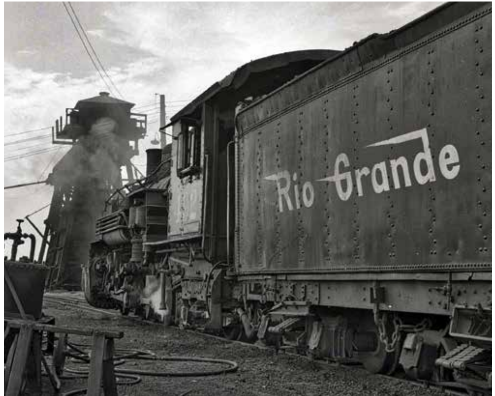
1958 Top: K-37 2-8-2 492 rides the turntable in Alamosa. Bottom: In the Alamosa engine terminal, a hostler fills 492's tender from a standpipe, then the locomotive heads for the coaling station.
