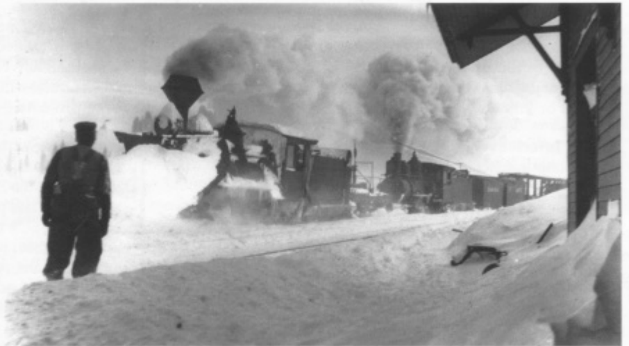
Railroading a century ago was hard, cold, dirty work. Here, a westbound freight arrives at Cumbres station, its thirty-ton Class 60 locomotive following a similar snowplow engine and flanger. As it proceeds, the train is clearing snow from the siding next to the main track. Photo by C. R. Lively from the Richard L. Dorman Collection of Narrow Gauge Photographs . (Caption by Vern Glover.)
