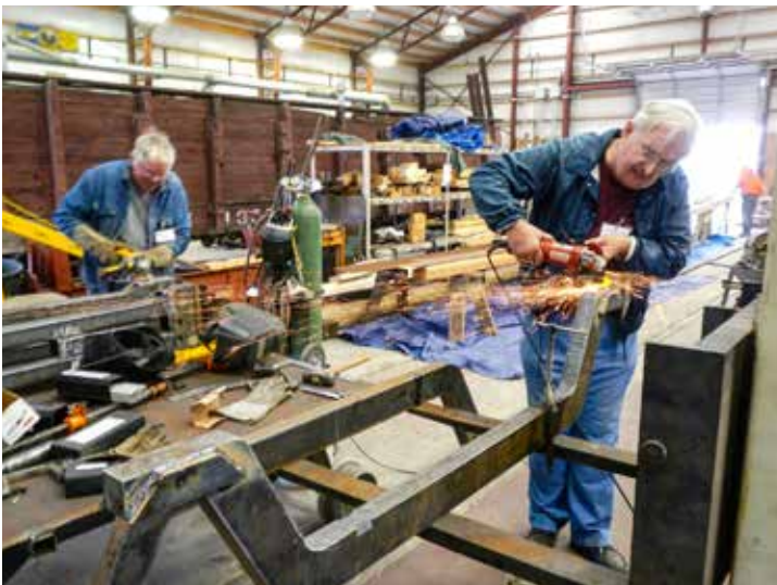
John Weiss, foreground, and Russ Hanscom, background are grinding welds on truck elements.
