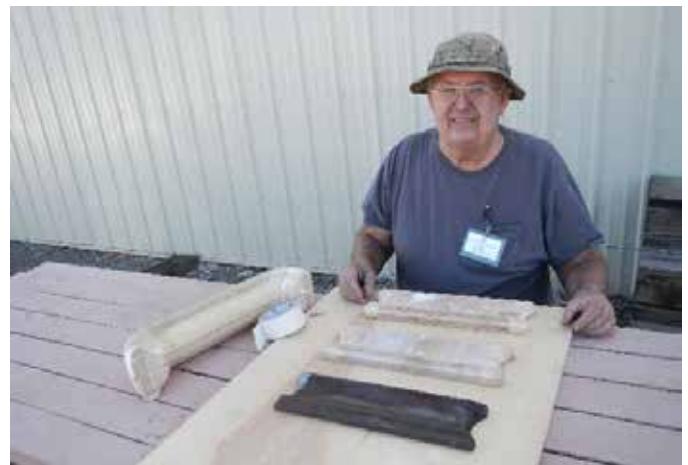
John Weiss is our Texas pattern maker. A worn out original part is in front. The new, carved wooden patterns will form the basis for the next batch of castings to be made later this year as funds become available.
