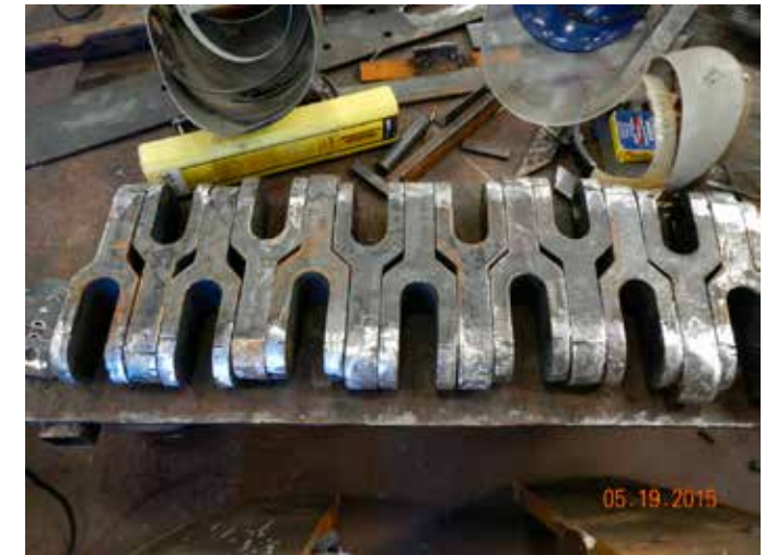
Newly built brake rod ends
