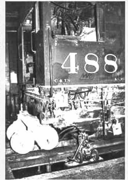
The new narrow-gauge shop trucks fabricated from standard-gauge ones. The shop trucks allow the engine to be moved while the lead and trailing trucks are being refurbished. (March 2001.)
